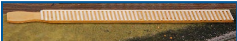
A jig Charlie made to assist in hand laying track
